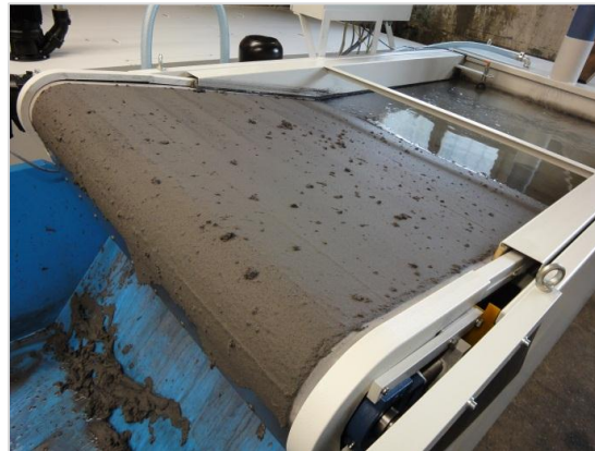
Picture 4: MAXFLOW belt filter made of self-cleaning stainless steel mesh from the GKD-CompactFiltration business unit.
