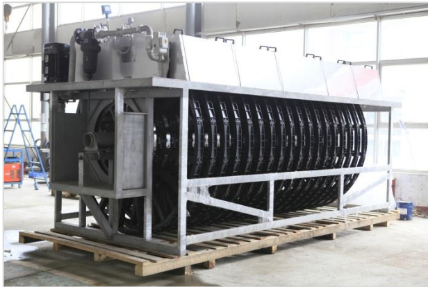
Picture 1: Disc filter for micro-screening with Optimized Plain Dutch Weave from the SolidWEAVE business unit.
