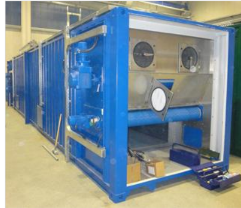
Picture 2: Compact belt dryer with Conducto® plastic fabric belt from the WEAVEinMotion business unit.
